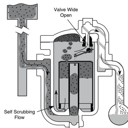
3. As the entering condensate starts to fill the bucket, the bucket begins to exert a pull on the lever. As the condensate continues to rise, more force is exerted until there is enough to open the valve against the differential pressure.
