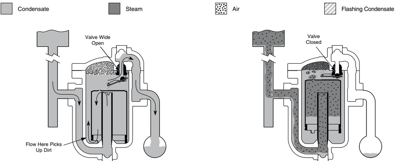
**1.** Steam trap is installed in drain line between steam-heated unit and condensate return header. On start-up, bucket is down and valve is wide open. As initial flood of condensate enters the trap and flows under bottom of bucket, it fills trap body and completely submerges bucket. Condensate then discharges through wide-open valve to return header.
